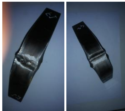
Specimen Image After Face Bending Test
