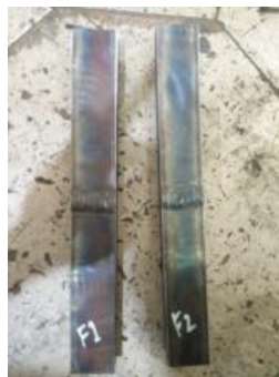
Images of Specimen F1 and F2 Before Face Bending Test
