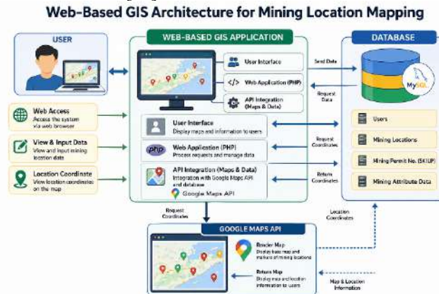
Figure 9. Web-Based GIS Architecture for Mining Location Mapping
