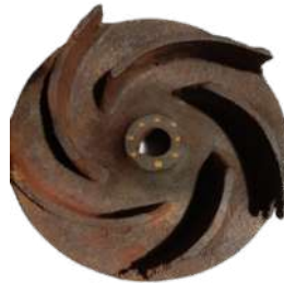
Figure 2. Overall failed impeller condition (front side)
