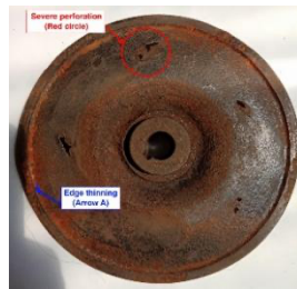
Figure 3. Failed impeller showing severe perforation (red circle), edge thinning (arrow A), and material loss at the outer diameter region.
