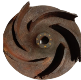
Figure 2. Overall failed impeller condition (front side)
