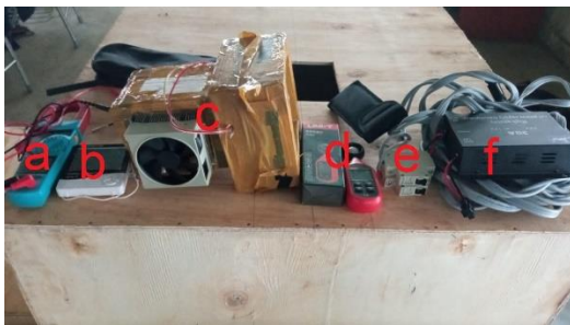
Gambar 2. Peralatan penelitian (a) Multi meter, (b) Thermometer, (c) Sistem pendingin
