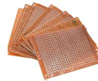
Gambar 7. Printed Circuit Board
