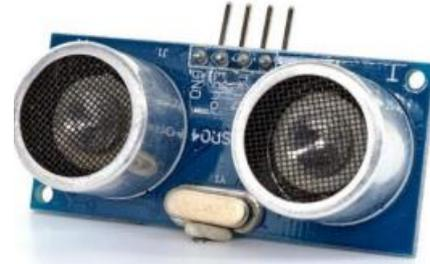
Gambar 1. Sensor ultrasonik HC-SR04
