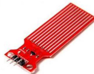
Gambar 2. Sensor *water level*
