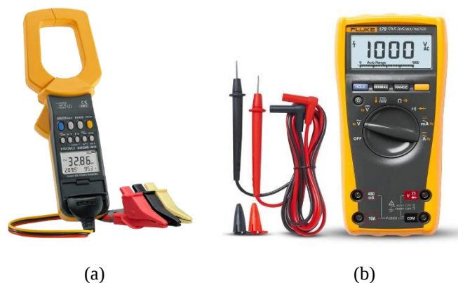
Figure 1. Measuring tools used : (a) Harmonics Analyzer and (b) AVO Meter
