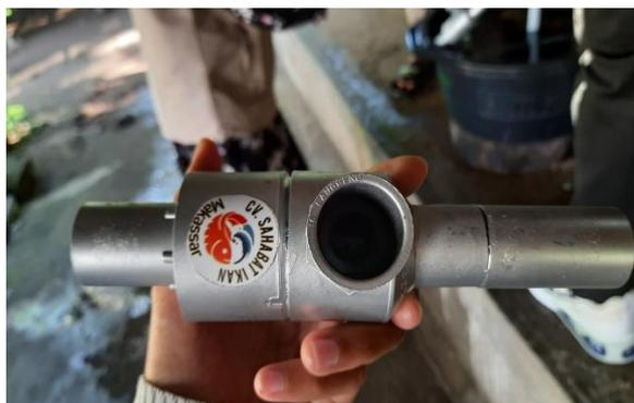
Gambar 1. Alat mikrobubble tipe venturi
