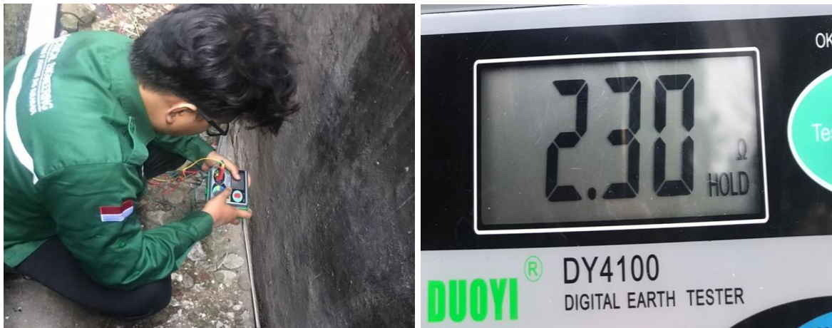
Figure 2. Measuring Soil Resistance Values with an Earth Tester
